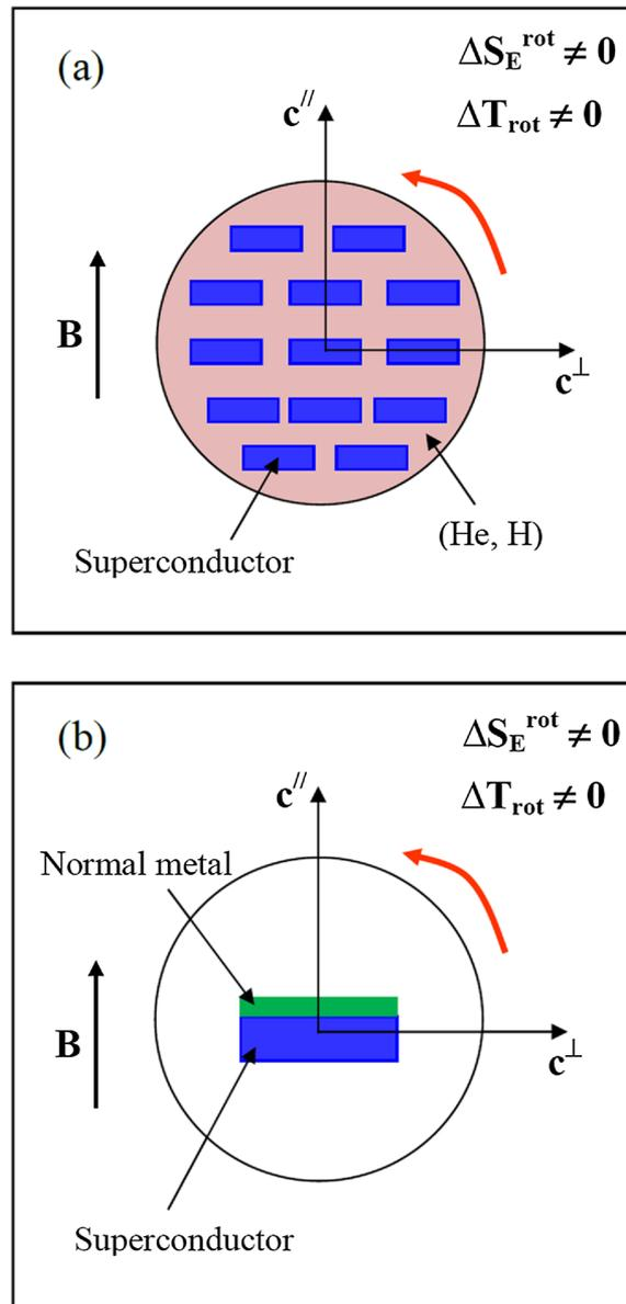
FIG. 3. Proposed cooling applications using superconducting materials as refrigerants and the principle of rotating them in the presence of a constant magnetic field. (a) The first design can be used for the liquefaction of helium and (b) the second design can be used for cooling down a normal metal.
